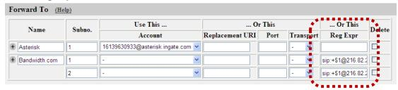
The Forward To attribute of the Dial Plan defines where to send the SIP traffic. A specific destination SIP URI address is defined to forward the call to. Here you may enter Regular Expressions for the Dial Plan, used to define where the Ingate should forward the request using the Dial Plan. Here you define GHM and use HAV.
