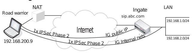
Additionally, for SIP to work over your IPsec connections, you require a tunnel under **IPsec tunnels** between the client and the **public** IP address of the Firewall/SIParator, i.e. the Local side address under **IPsec Peers**. This requires a Phase 2 connection in the client (The Greenbow) also.
