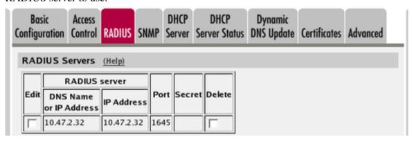
You must also select which IP address the Firewall/SIParator should use when contacting the RADIUS server.
