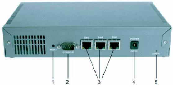
The firewall/SIParator can be rebooted in several ways. You can press the RESET button (item 1 in the figure) on the back (requires a pencil or other thin device), or simply disconnect the power cord and connect it again.
